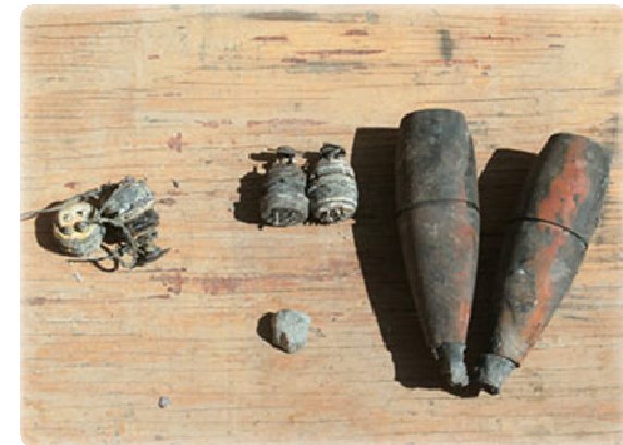
Burned-out 60mm M768 projectiles recovered from MRAP
